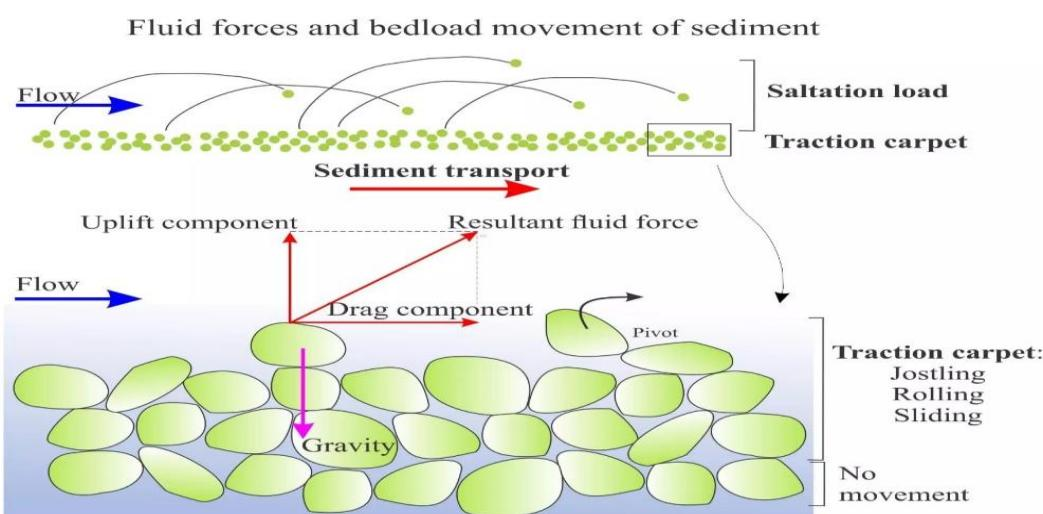
*Figure-23: Bedload Movement of Sediment*
