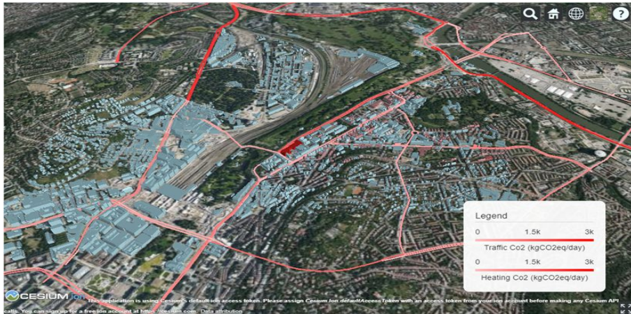
CO2 Emissions Traffic and Building Sector H. Ebrahim: Concept and Evaluation of an Urban Platform for Interactive Visual Analytics, Master HFT Stuttgart
