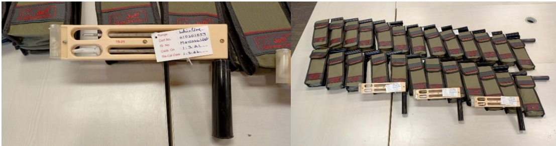
Figure 8:Reference Travelling Standard Whirling Psychrometer.
