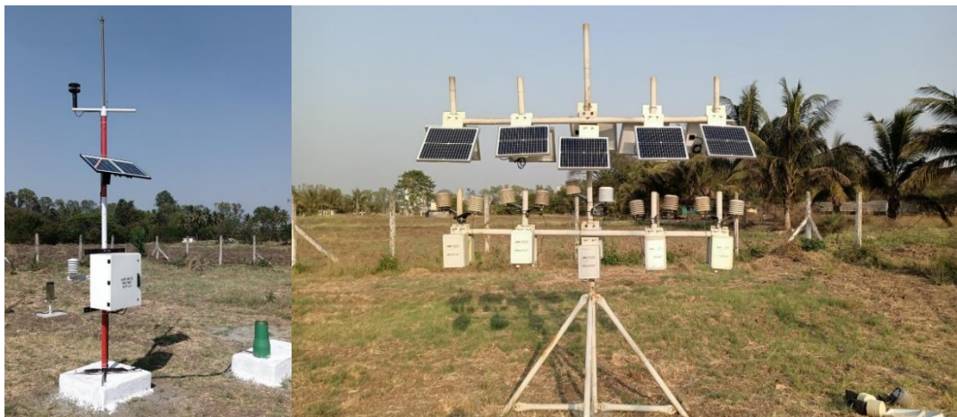
Figure 6: Sensors collocated with Reference Grade AWS for field calibration and comparison on field
