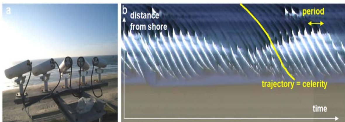
Figure-10: Coastal video monitoring: description of applications; (a) 5-camera system for Biscarrosse (France); (b) Spatial-temporal post- processed image showing wave dynamics. The image is generated from the high frequency acquisition of a cross-shore array of pixels. (source: . Marchesiello et al. / Ocean Modelling 96 (2015) 36–48).
