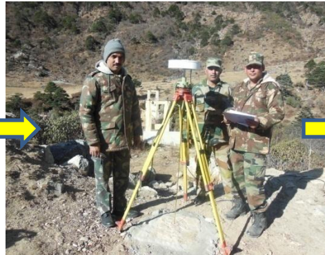
PLACING OF MARKERS ON GROUND & GPS OBSN
