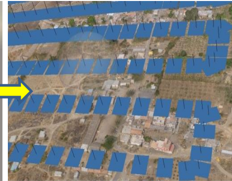
ALIGNMENT OF PHOTOS ON SOFTWARE
